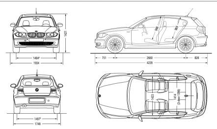
All dimensions in millimetres (shown here the BMW1 Series 5-door). Luggage compartment capacity approx. 330 to 1,150 litres (11.7 to 40.6 cu ft).
